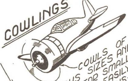
VARIOUS SIZES AND SHAPES FOR SMALL MODELS CAN EASILY BE MADE FROM DISCARDED BOTTLE CAPS
